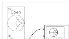
Circuit 14. Open Display S11 Smith Chart, START=50kHz, STOP=1000MHz
